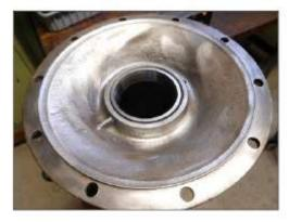
The inside of the axle housing should be smooth
