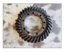
Teeth broken off the ring gear
